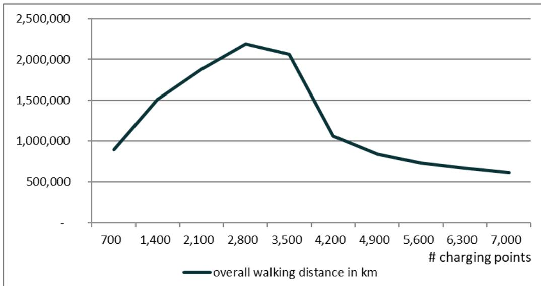
Figure 9: Impact of the number of the charging points on the overall walking distance
