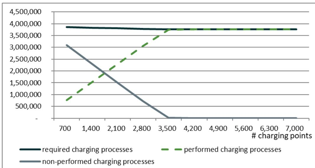
Figure 8: Impact of the number of charging points on the required, performed and non-performed charging processes
