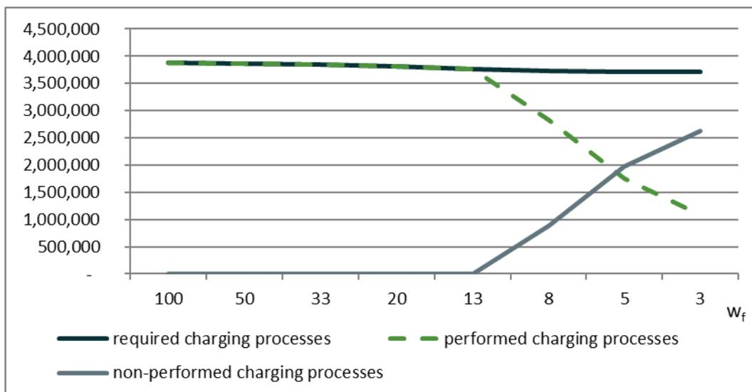
Figure 5: Impact of the charging duration on the required, performed and non-performed charging processes
