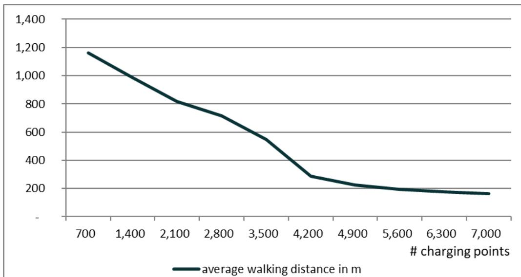
Figure 10: Impact of the number of the charging points on the average walking distance per performed charging processes
